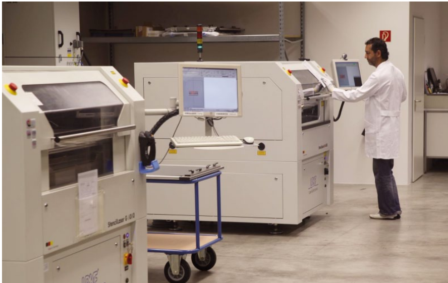
FIGURE 2: Having invested 300,000 euro in a high-speed system from LPKF, photocad relies on the latest laser cutting technology for its SMD stencils. The system is specifically designed to produce high-precision openings, while at the same time also speeding up the operating procedure. (Source: photocad GmbH & Co. KG)
