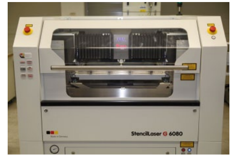
FIGURE 3: The new laser cutting system is equipped with a special control system that scans the stencil openings in real time and changes the parameters if necessary – without shutting down. (Source: photocad GmbH & Co. KG)
