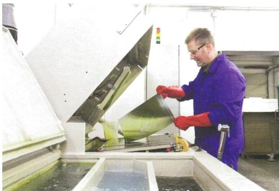
Stencil electropolishing in the machine ensures placement reliability
