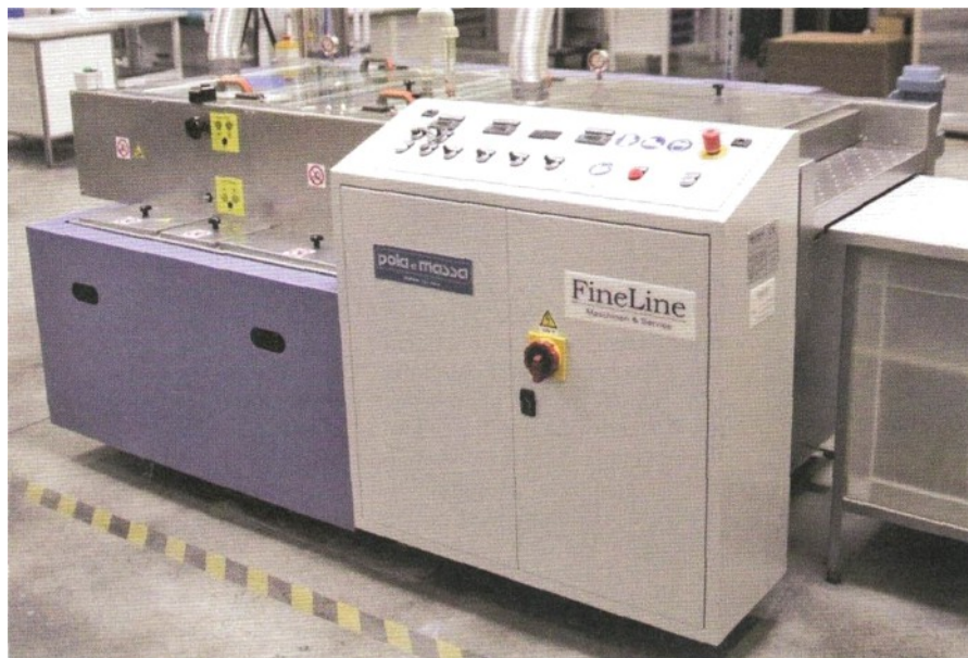
Continuous washing system: precise cleaning as a prerequisite for exact apertures
